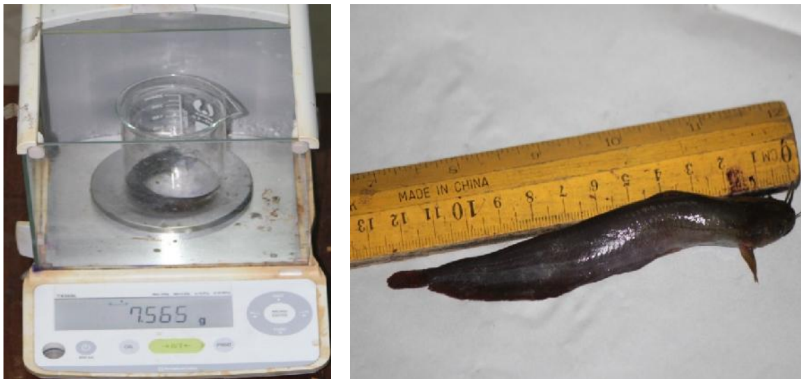
Plate 2.5: Weight and length were measured by using an electric balance and a centimeter scale
