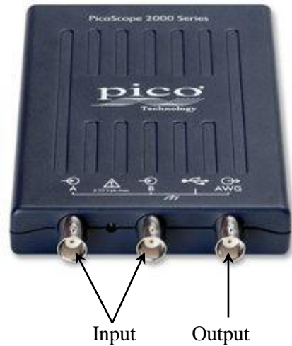
Figure 3-20 Portable oscilloscope (Picoscope) used for data acquisition.
