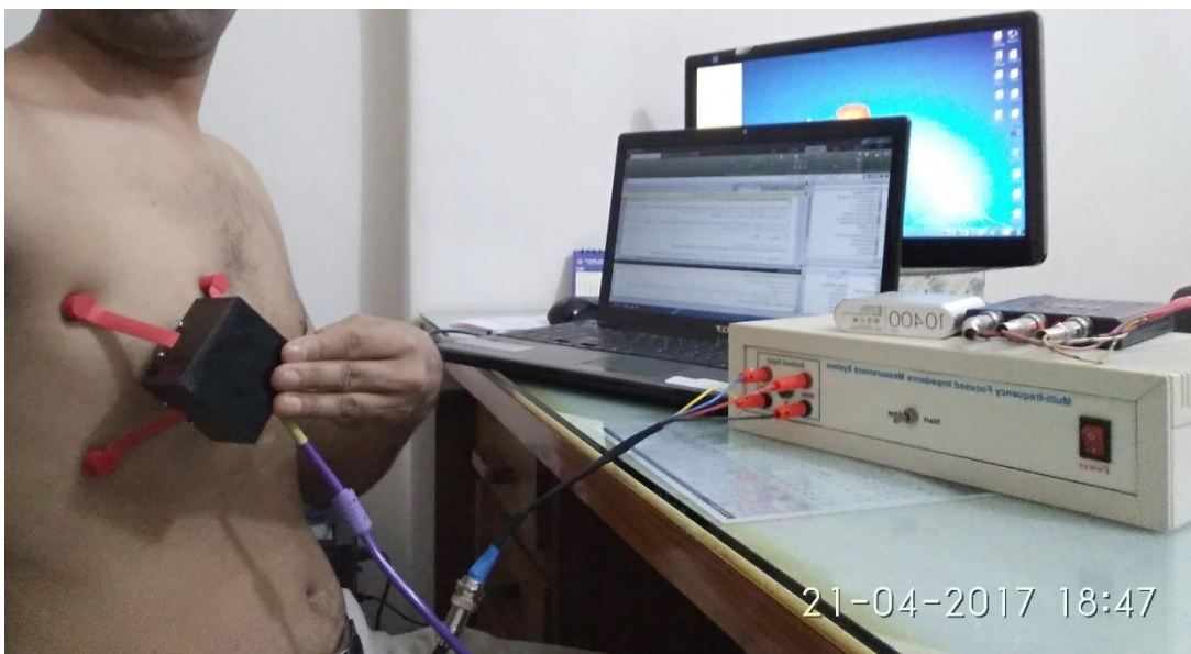
Figure 4-55 Experimental setup for measurement of focused impedance from human subject using multi-frequency FIM system made as a part of the present work. The electrodes are mounted on a hand held portable probe.
