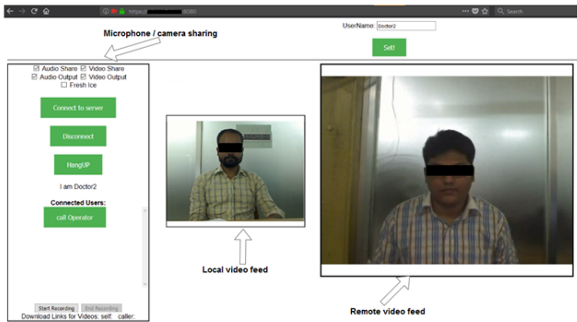
Fig. 6.3 Web-based real-time multimedia communication user-interface integrated into the TMS
