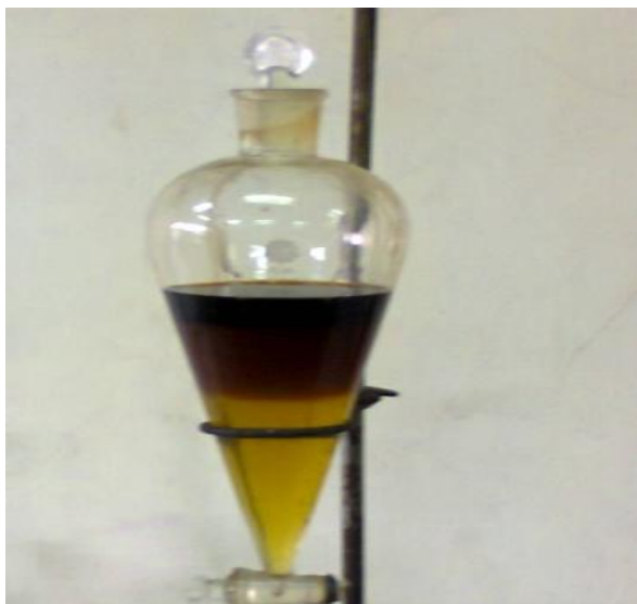
Photo 173. Solvent-solvent partitioning of crude extract
