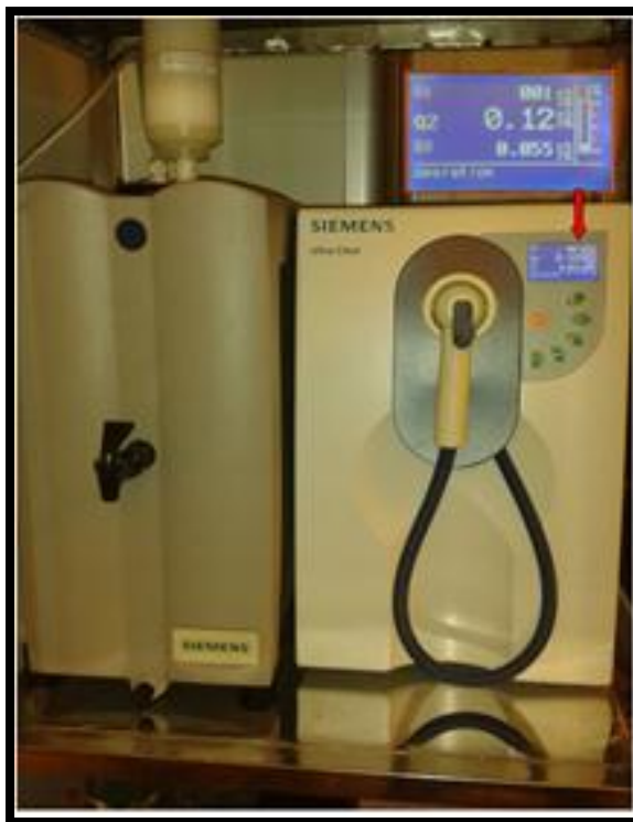
Figure App 1: Front side view of De-ionized water plant.
