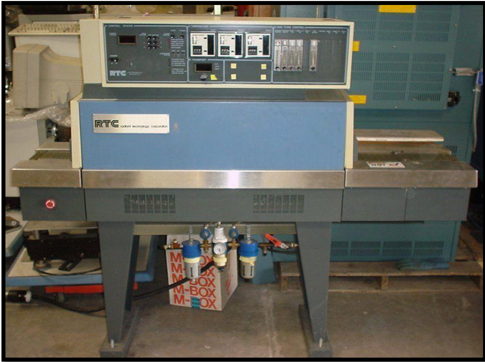
Figure App 10: Front side view of RTA belt furnace
