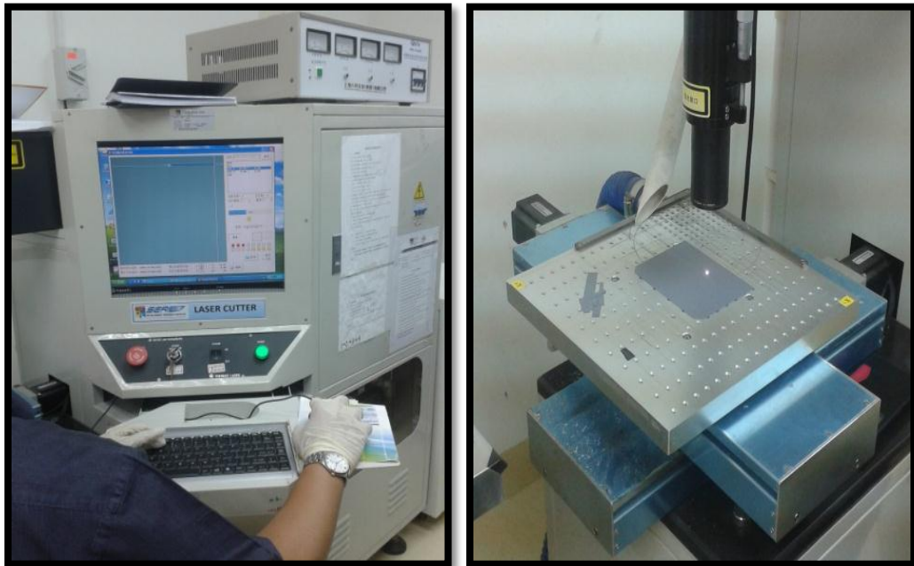
Figure App 2: (a) Front side view of laser cutter (b) Silicon wafer under the laser cutter
