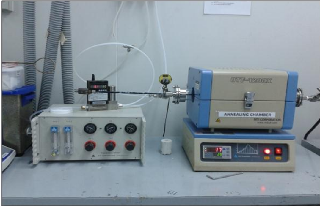
Figure 5.13 Diffusion Process inside the annealing furnace
