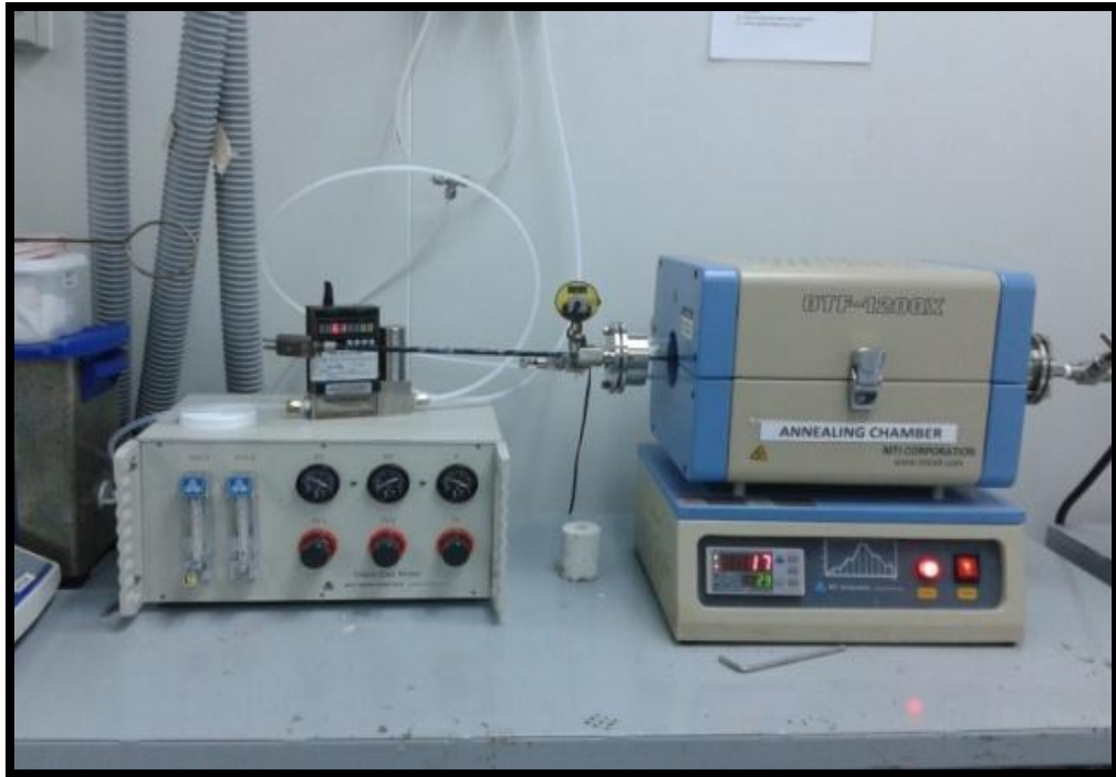
Figure App 8: Front side view of annealing furnace
