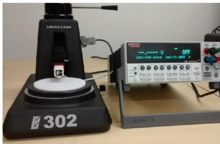
Figure App 20: Image of Sun four point probe instrument for sheet resistivity measurement [15].
