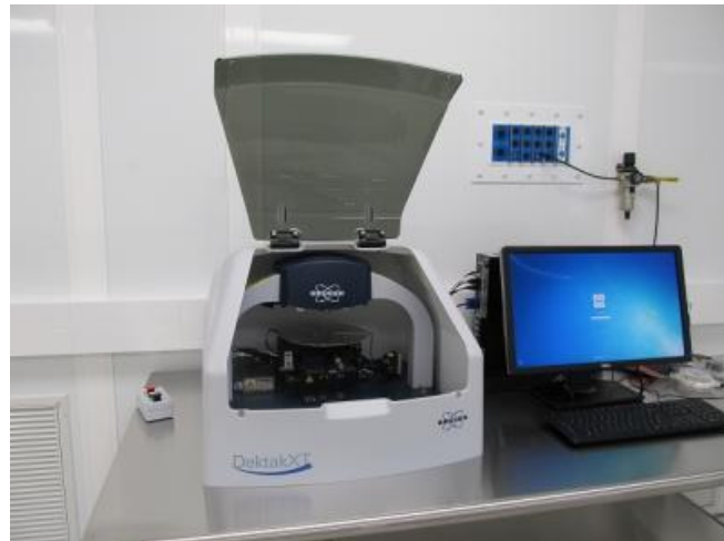
Figure App 9: Image of DektakXT stylus surface profiler for thickness measurement of silicon film [13].
