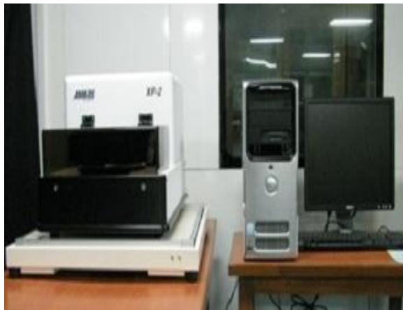
Figure App 7: Image of Ambios stylus surface profiler for thickness measurement of silicon film.
