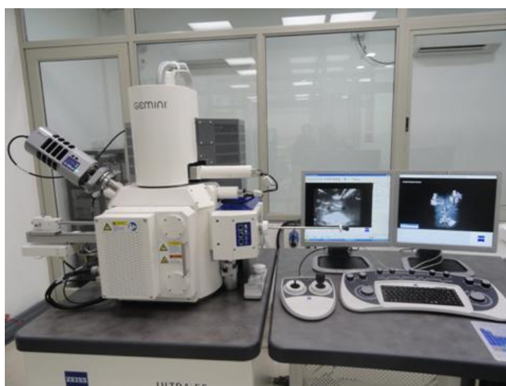
Figure App 14: Image of scanning electron microscope with oxford energy dispersive x-ray (EDS) unit [15].
