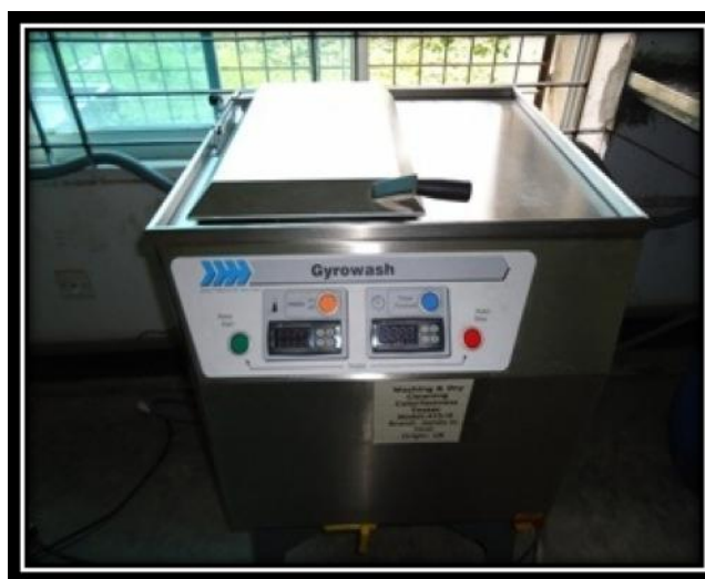
Figure 3.6: Wash fastness tester (Gyrowash) for the assessment of color fastness to washing of dyed fabric.
