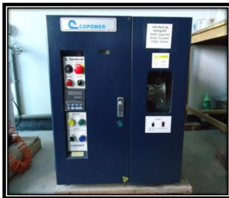
Figure 3.3: Sandolab Infrared lab dyeing machine for the pretreatment and dyeing of cotton fabric.
