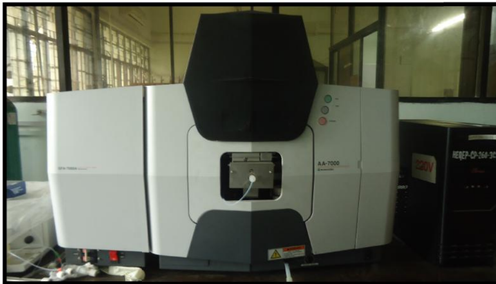
Figure 3.1: Atomic absorption spectrophotometer for the measurement of heavy metals in wastewater
