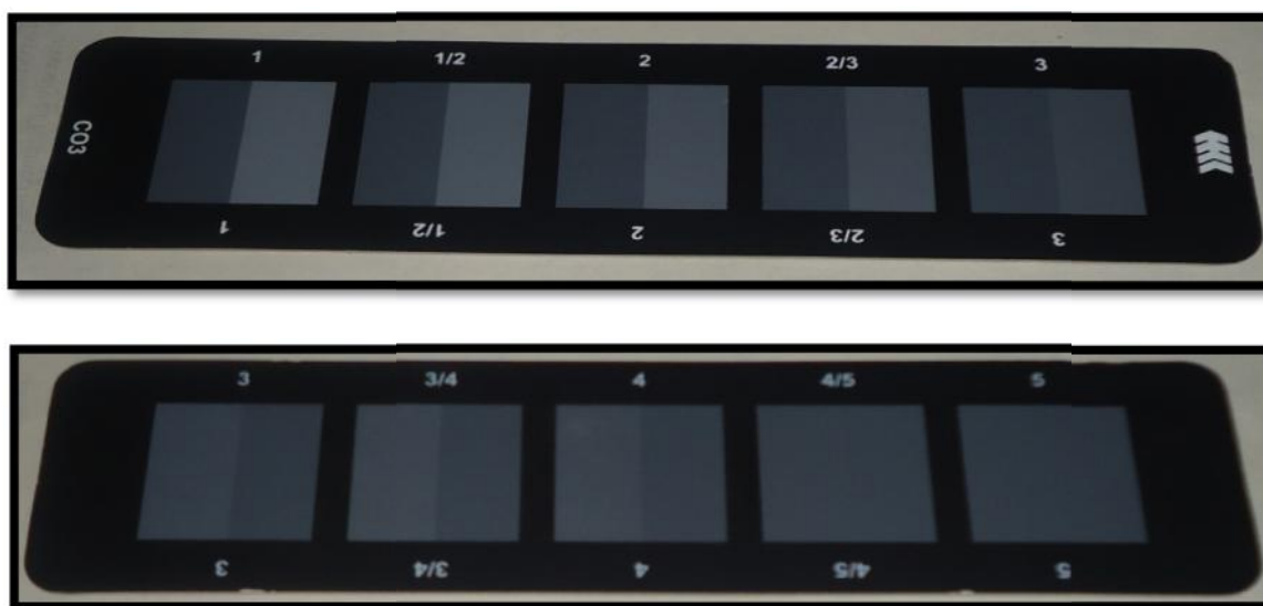
Figure 3.7: Color change grey scale for the evaluation of color fastness properties of dyed fabric
