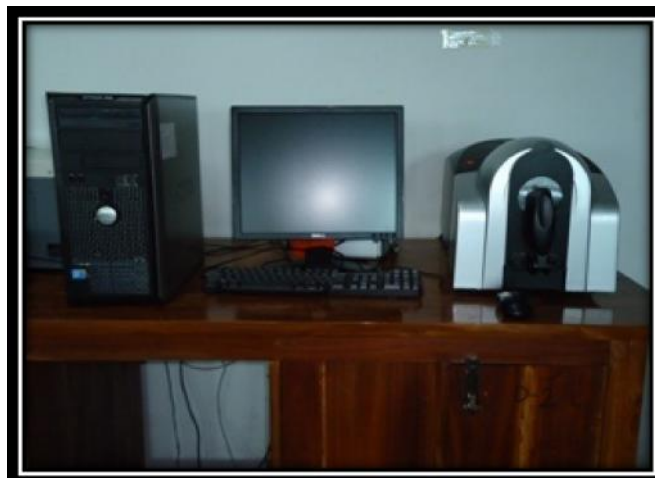
Figure 3.5: Spectrophotometer (Data Color 650) for the measurement of color and whiteness of fabric.
