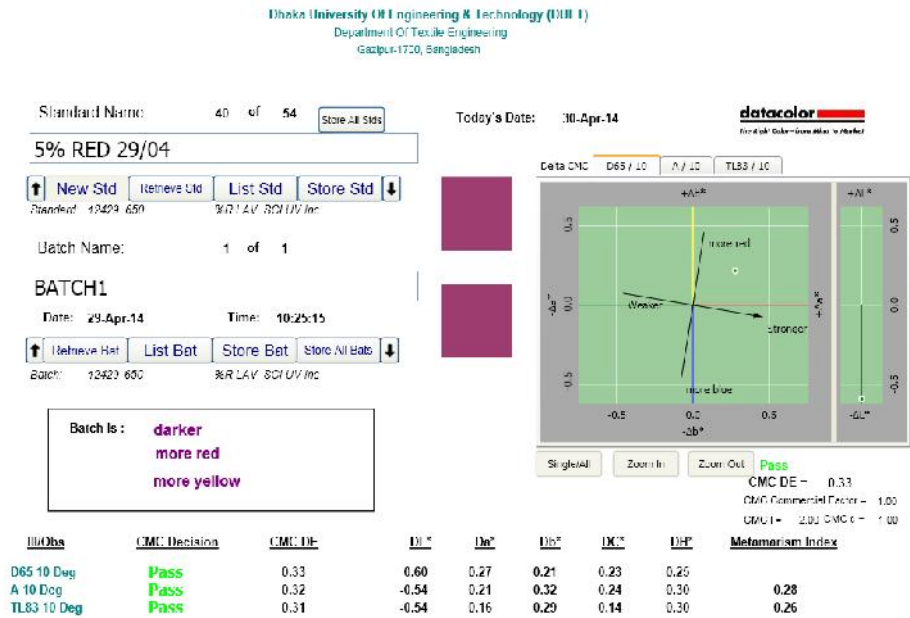
Figure D.1: Color matching of fabrics dyeing in fresh and irradiated water with Novacron Red FN 2BL at 5.0% shade.
