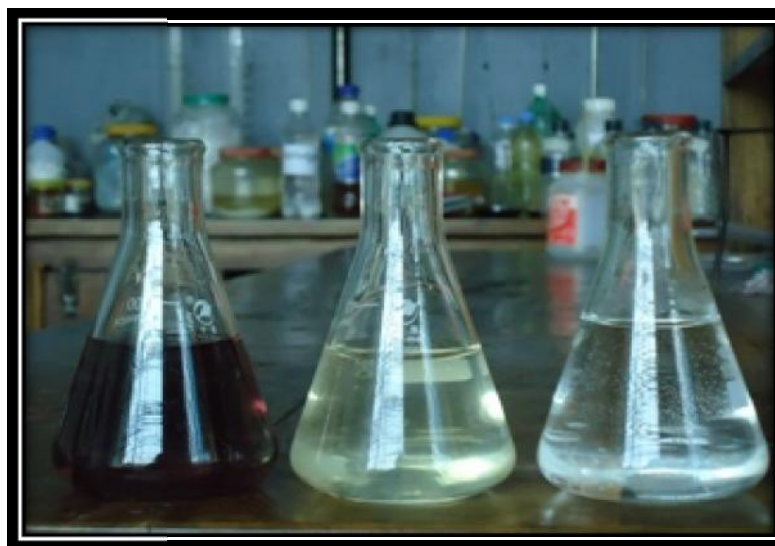
Figure 4.1.3: Appearance of raw and gamma irradiated (at 12 kGy radiation dose) wastewater with respect to the fresh water .
