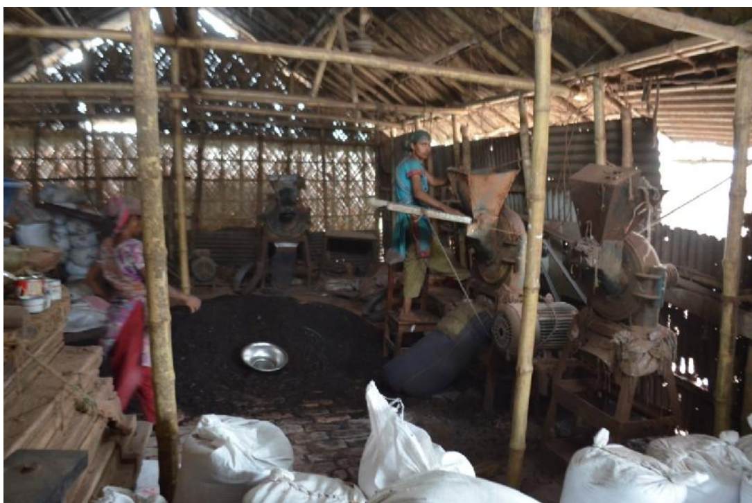
Figure 15: Grinding of dried protein concentrate.
