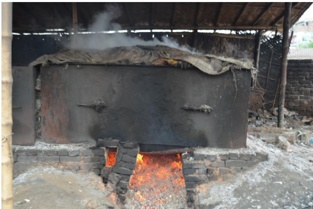
Figure 14: Boiling of chrome shaving dust with H_2SO_4 .
