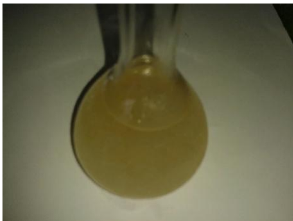
Figure 21: Collagen Hydrolysate prepared by MgO and trypsin.
