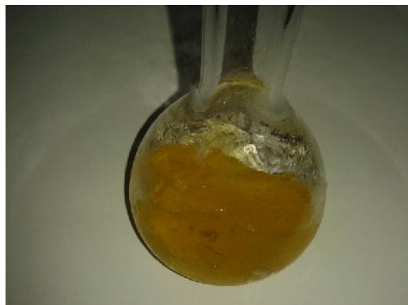
Figure 22: Collagen Hydrolysate prepared by CaO and trypsin.
