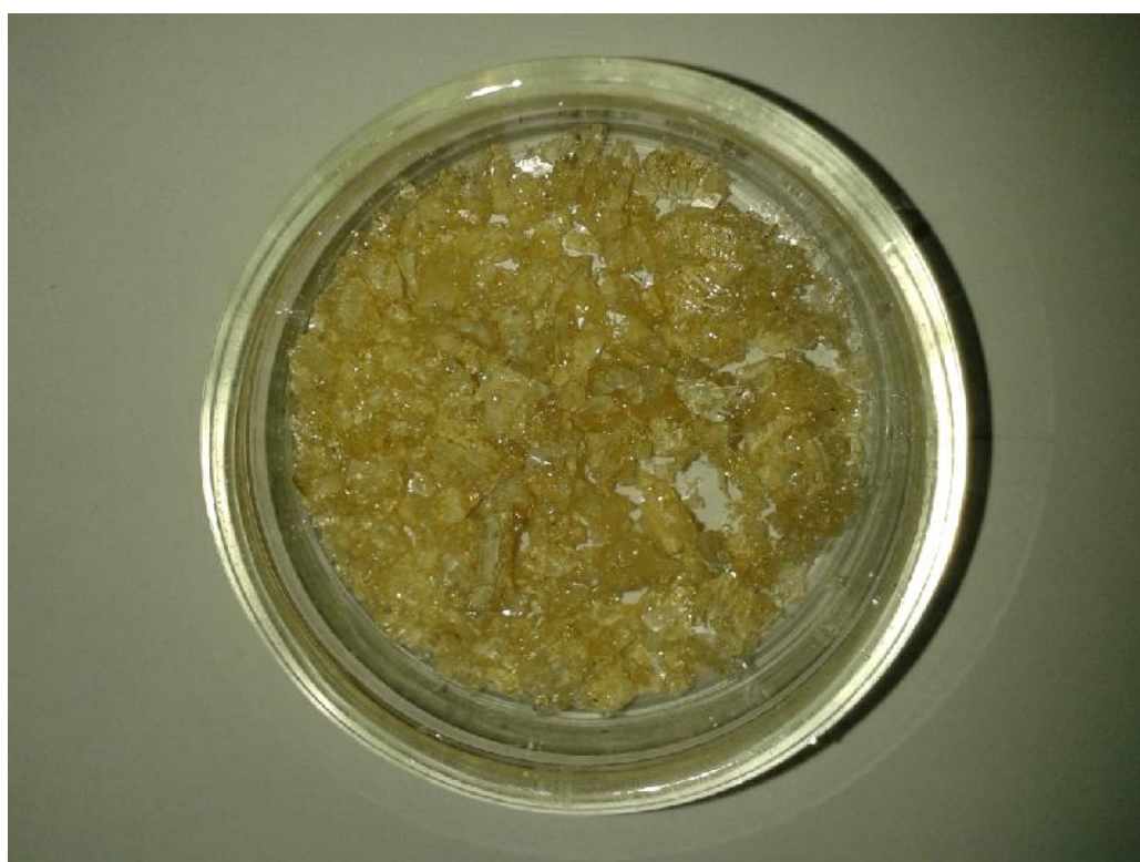
Figure 23: Freeze dried Collagen Hydrolysate prepared by MgO and trypsin.
