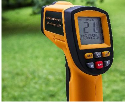
Figure 3.1.3: Infrared (IR) thermometer. A non-contact type thermometer gun. It can measure object temperature by calculating the amount of infrared radiation emission.
