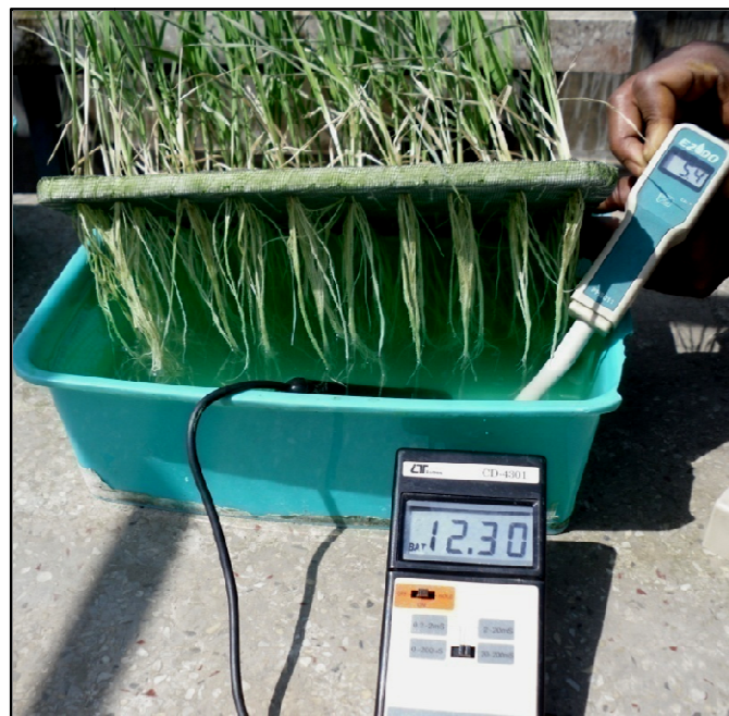
Fig. 3.9: pH ( 5\pm 0.5 ) and EC ( 12\pm 0.5 ) \text{dSm}^{-1} for seedling stage screening in hydroponics? culture were checked daily by pH meter and EC meter.
