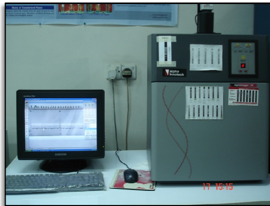
Fig. 3.5: Alpha Innotech gel documentation system
