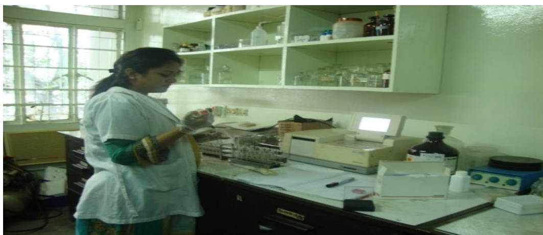
Figure 2.6.c: Pipetteing working reagent in test tubes.
