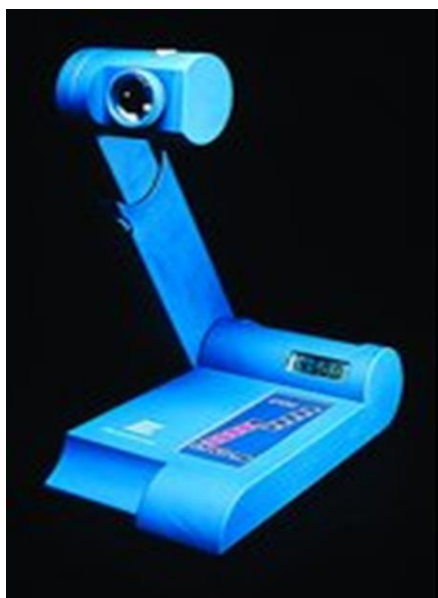
Figure 3.6 Electro thermal melting point apparatus.
