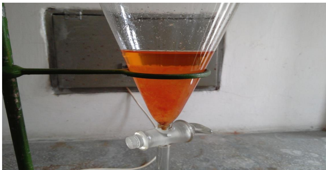
Figure 4.5 Extraction of tomato paste using ethyl acetate (EtOAc) solvent.
