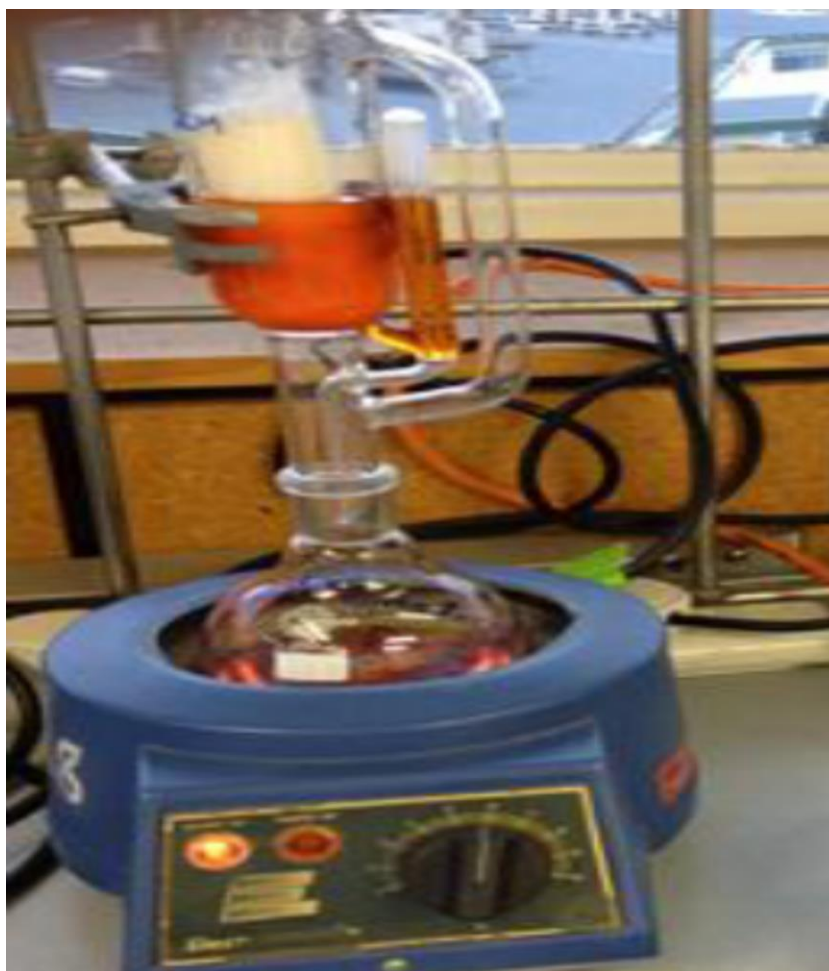
Figure 4.15 Soxhlet Extraction of tomato paste using ethyl acetate (EtOAc)
