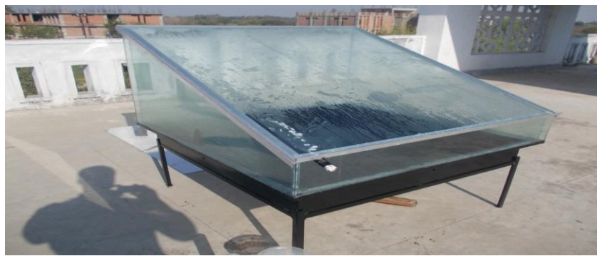
Fig-36: Photograph of the modified design single slope solar still
