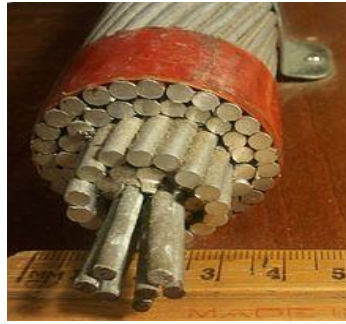
Figure 2.25: Sample cross-section of high tension power line, showing 7 strands of steel surrounded by 4 layers of aluminum [10]
