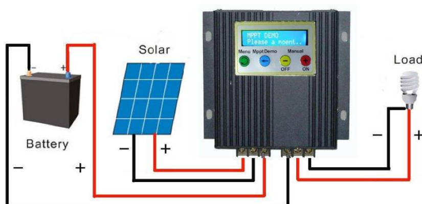
Figure 2.21: Charge controller with Solar panels, battery and loads [14]
