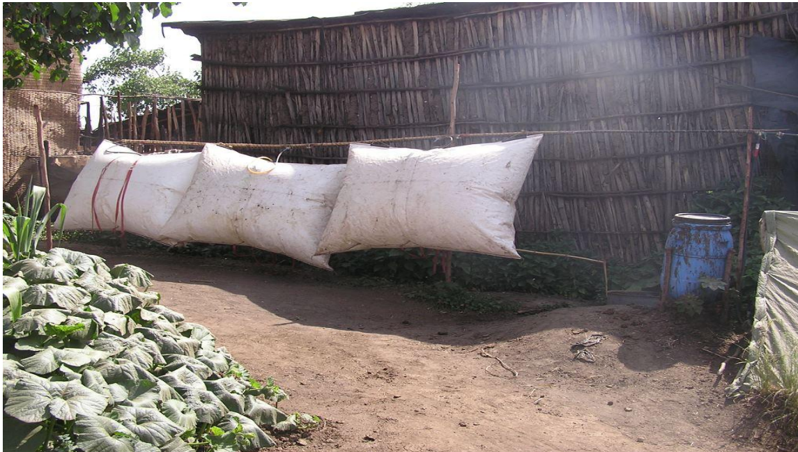
Figure 27: Portable biogas plants are installed in village [52]
