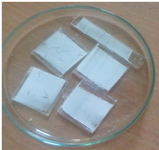
Figure 6: Fully prepared Titanium di-oxide based photo anodes
