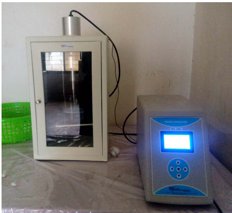
Figure 5: Ultrasonic Cleaning of ITO glasses using cleaning solvent in sonicator
