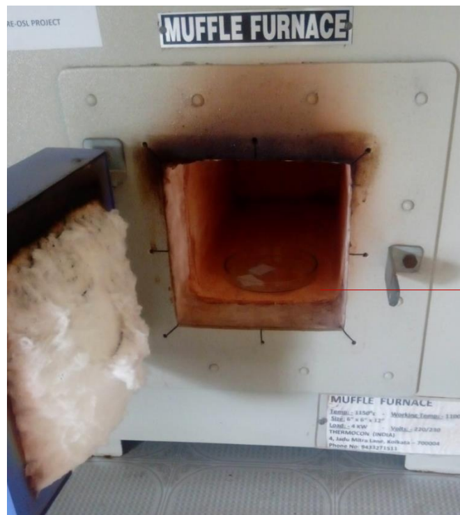
Figure 19 ITO Glass after Annealing in Muffle Furnace
