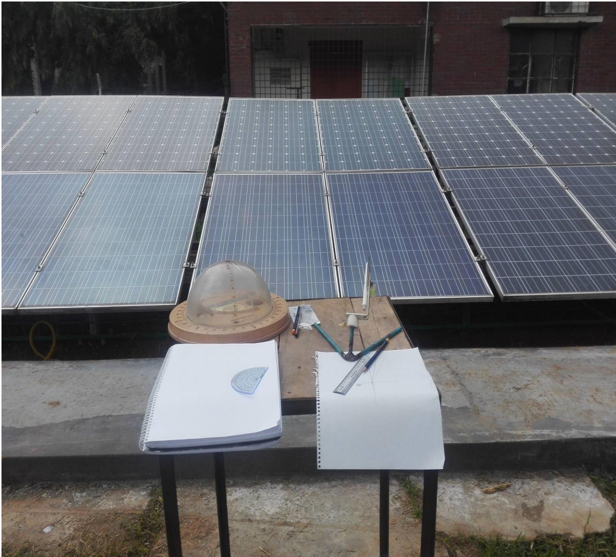
Fig – 8.2: Instruments used for drawing of horizon profile diagram on sun-path diagram.
