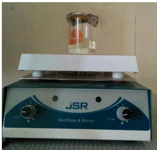
Figure 14 TiCl 4 solution being stirred on a stirrer.
