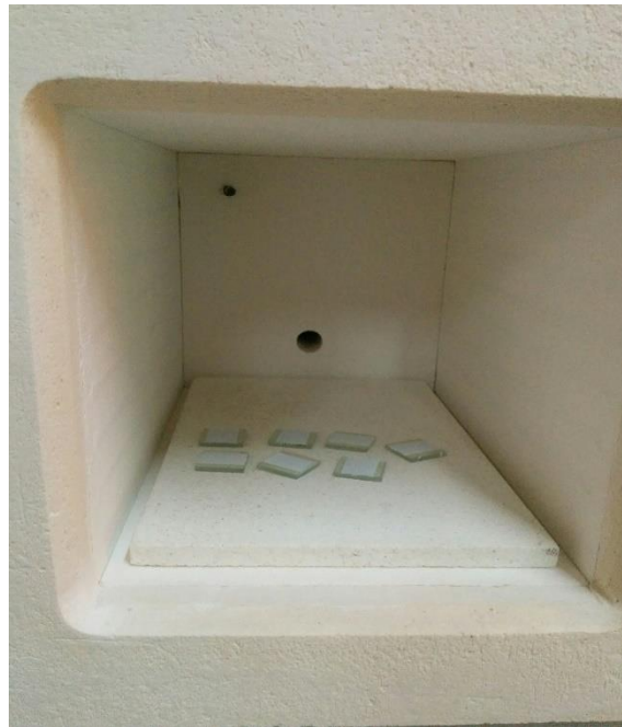
Figure 13 Photoelectrode in a muffle furnace
