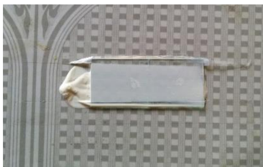
Figure 12 Applied TiO 2 paste on the ITO glass using glass
