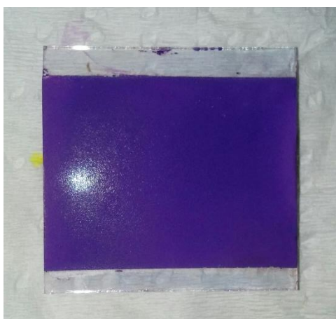
Figure 16 A photoelectrode dyed with blackberry dye.
