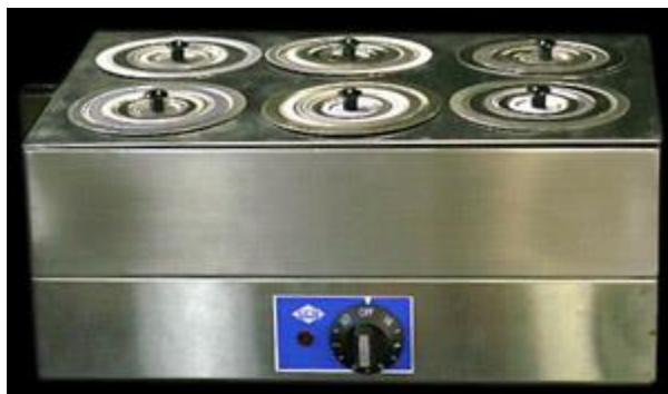
Figure 15 Water bath to maintain continuous temperature while coating.
