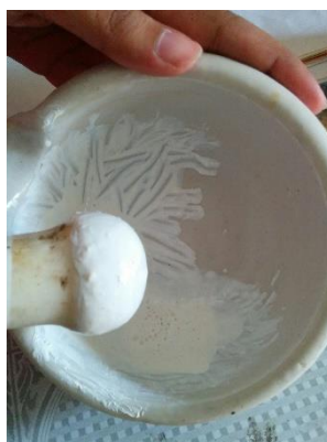
Figure 11 Titanium dioxide paste preparation in a mortar
