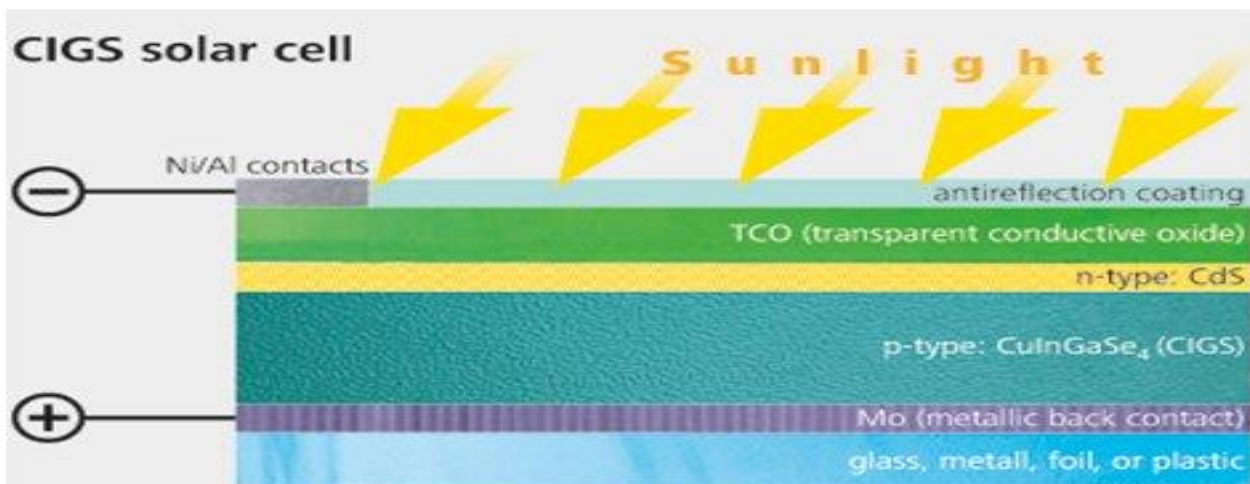
Figure 2.9 Copper indium gallium selenide solar cells [13]
