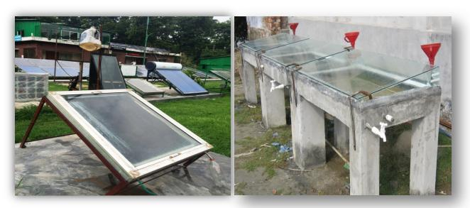
Figure 4.8- Fabric Type Solar Still (FSS) and Basin Type Solar Still (BSS)
