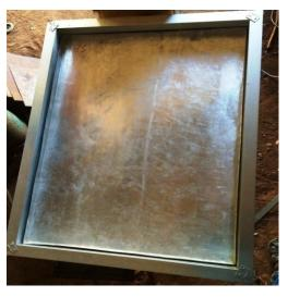
Figure 3.10- Assemble the aluminum tray with the rectangular frame
