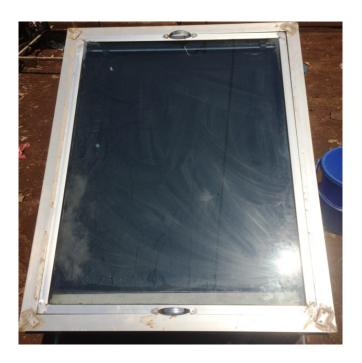
Figure 3.13- Setup the top glass cover
