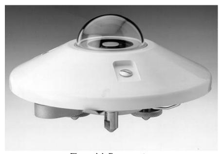
Figure 4.4- Pyranometer
