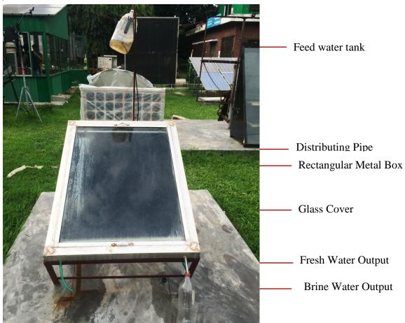
Figure 3.1- Solar Still desalination with fabric absorber
