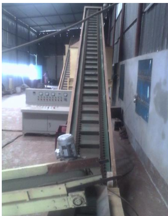
Figure 7.6: Ready pellet is going to cooling unit
