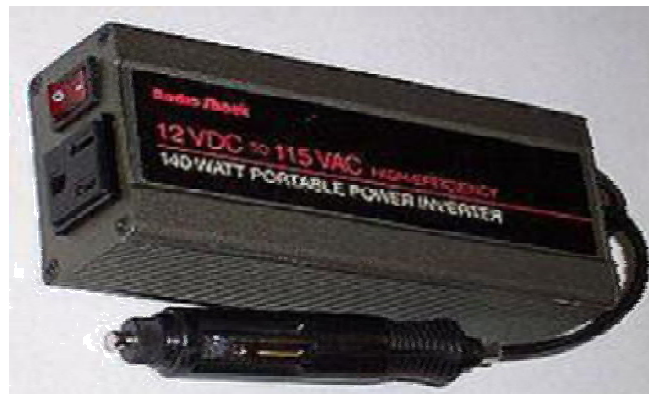
Figure2.3: Inverter designed to provide 115 VAC from the 12 VDC source provided in an automobile. The unit shown provides up to 1.2 Amps of alternating current, or just enough to power two sixty watt light bulbs
