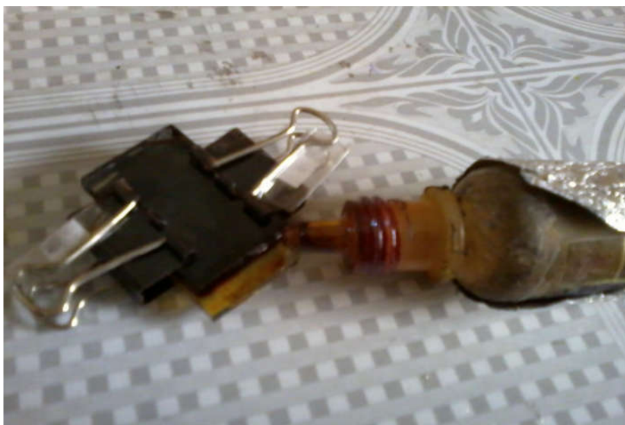
Figure 5-13 Electrolyte is pouring in the prepared DSSC
