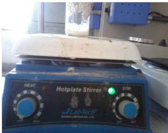
Figure 5-4 Magnetic Stirring of the solution at MAGNETIC STIRRER HOTPLATE
