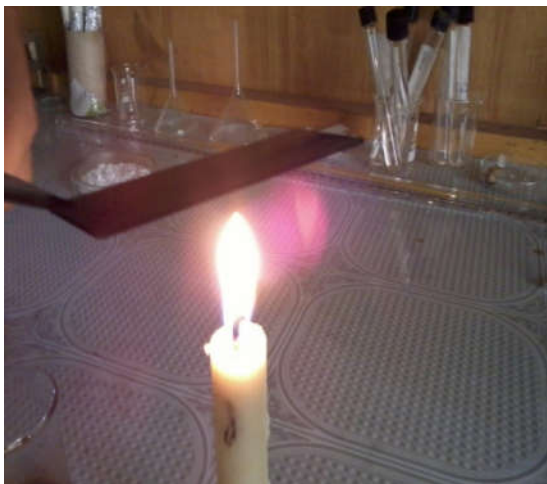
Figure 5-12 Prepared Counter Electrode made by tip of Flame
