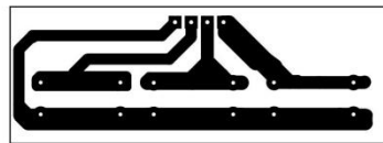
Figure 31 PCB of the I-V tracer circuit
