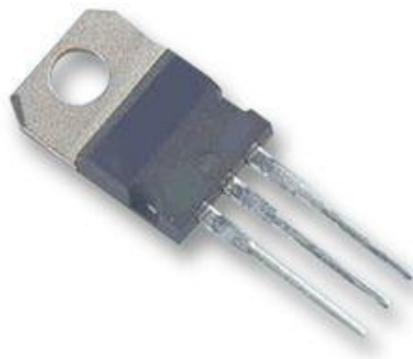
Figure 16 N-Channel Power MOSFET RFP70N06
