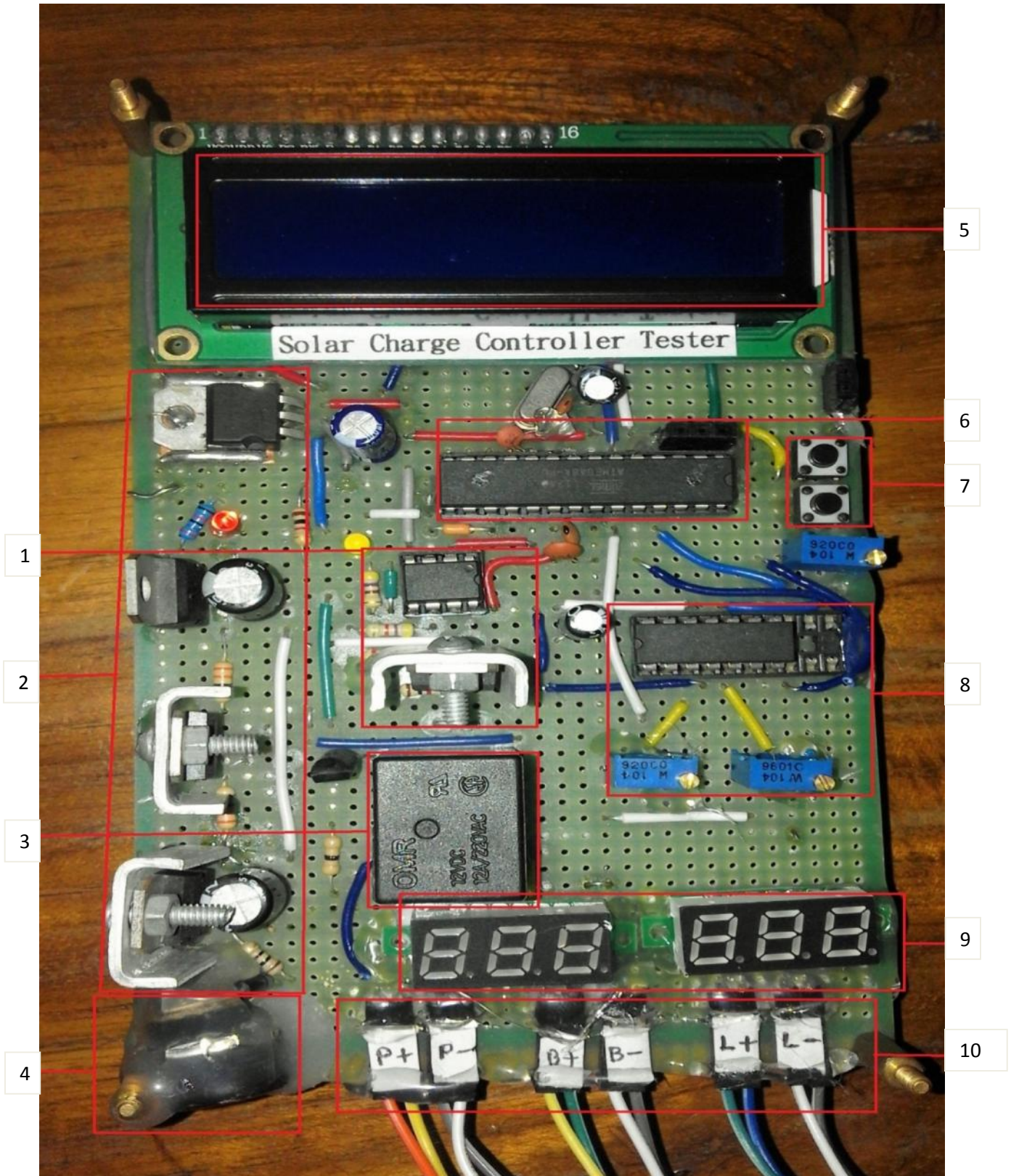
Figure 19 Charge Controller testing Unit
