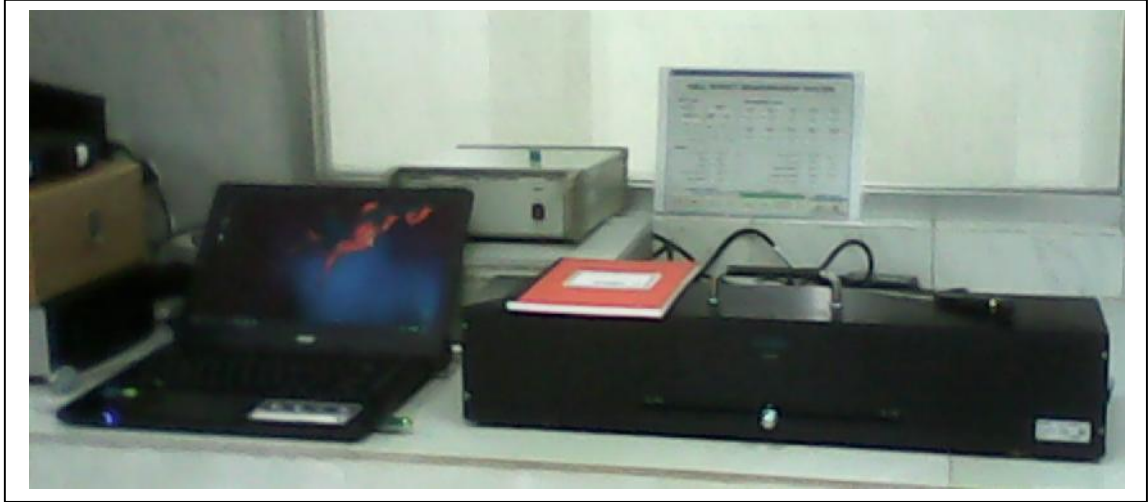
Figure 7.5: Hall Effect Measurement of 10 times deposited layer using ECOPIA HMS-3000
