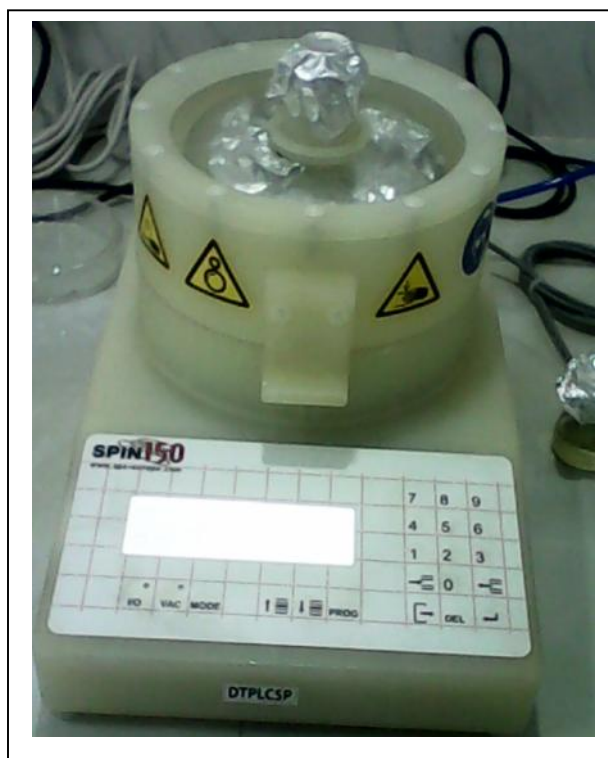
Figure 5.4: Spin Coating of the slides with DTPLCSP SPIN150 Spin coater
