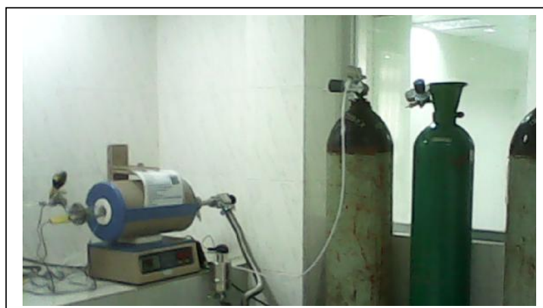
Figure 5.6: Air annealing of samples with machine DTLCSP C-1000
