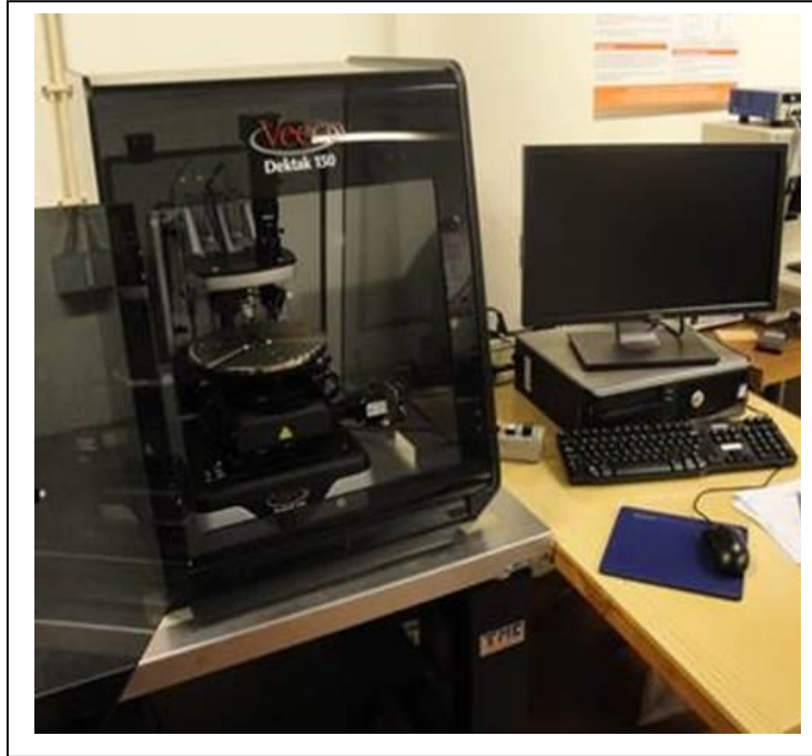
Figure 7.1: Stylus Surface Profilometer, Model: Detak-150
