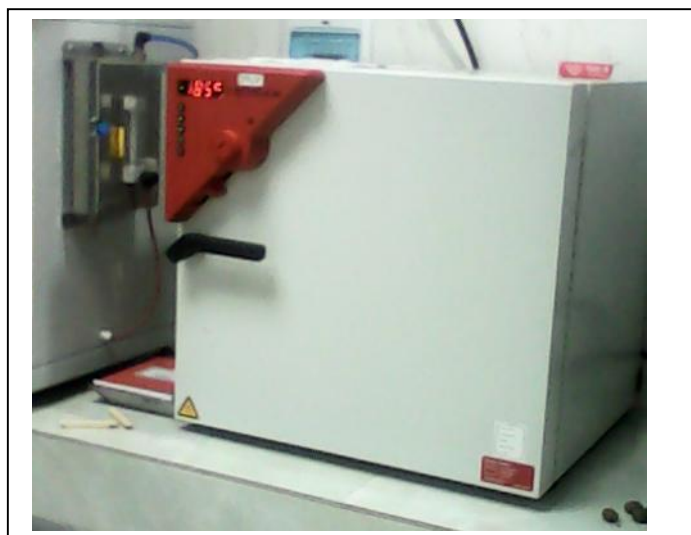
Figure 5.5: Ageing at 300°C in DTPLCSP BINDER machine
