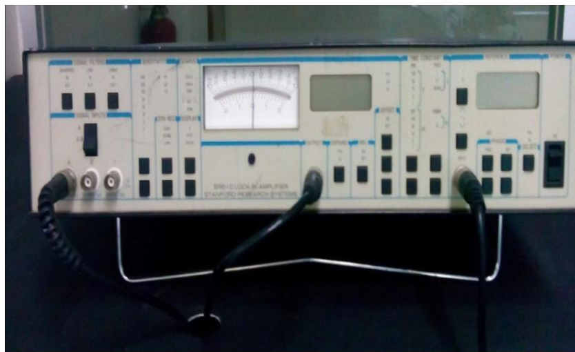
Figure 5.5. Stanford research 510 lock-in amplifier.
