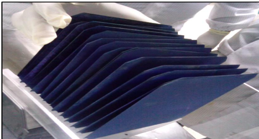
Figure 3.7. The phosphorus doped silicon wafer [3]
