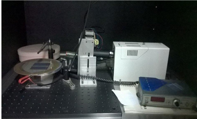
Figure 4.6. SPV Measurement System.
