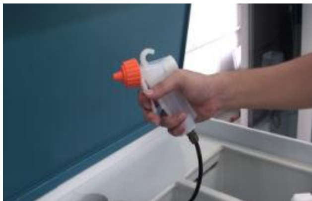
Figure 3.5. Compress air gun for wafer drying [6]
