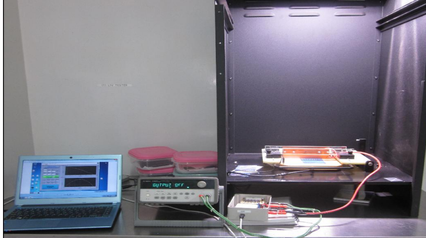
Figure 4.4. LIV measurement System [2]
