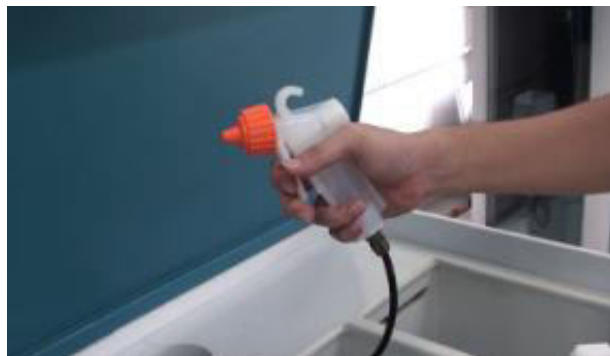
Figure 3.5. Compress air gun for wafer drying
