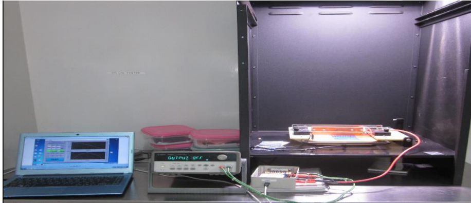
Figure 4.4: LIV measurement System
