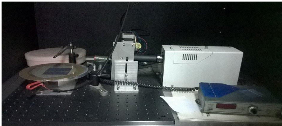
Figure 4.7: Picture of SPV Measurement system.
