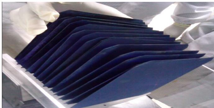
Figure 3.7. The phosphorus doped silicon wafer
