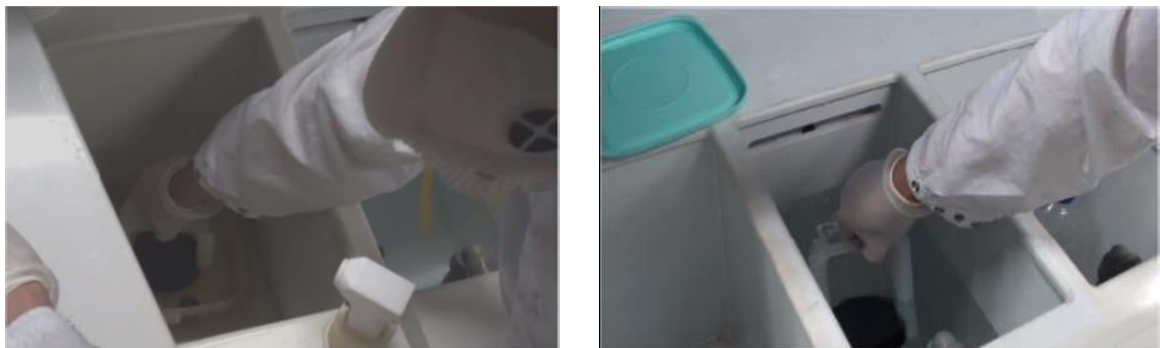
Figure 3.2.RCA cleaning process: DI water dip(left),cleaning process: Nitric Acid solution(Right)
