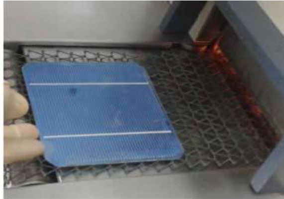
Figure 3.10. Contact firing at RTC furnace
