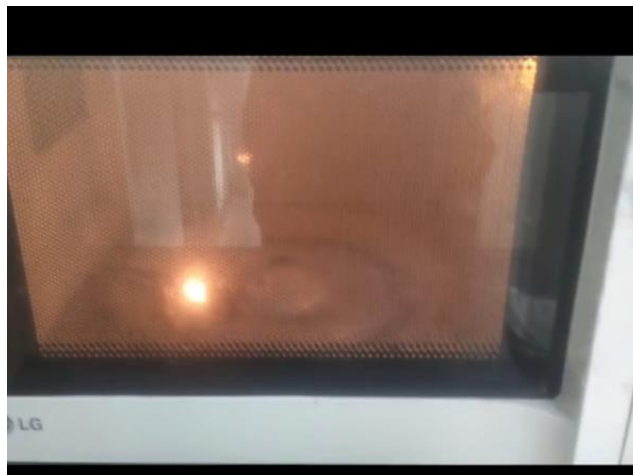
Figure-4.3: Microwave exfoliation of Graphene using microwave arc radiation
