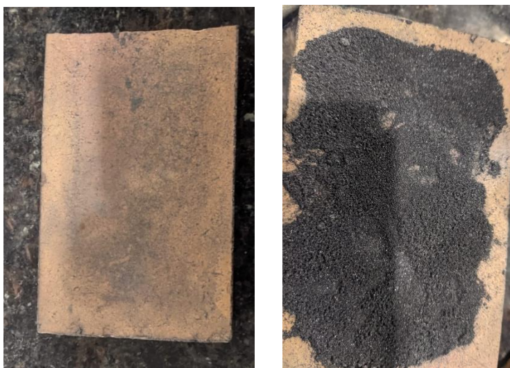
Figure-4.5. The ceramic tiles that were used for the exfoliation of intercalated graphite
