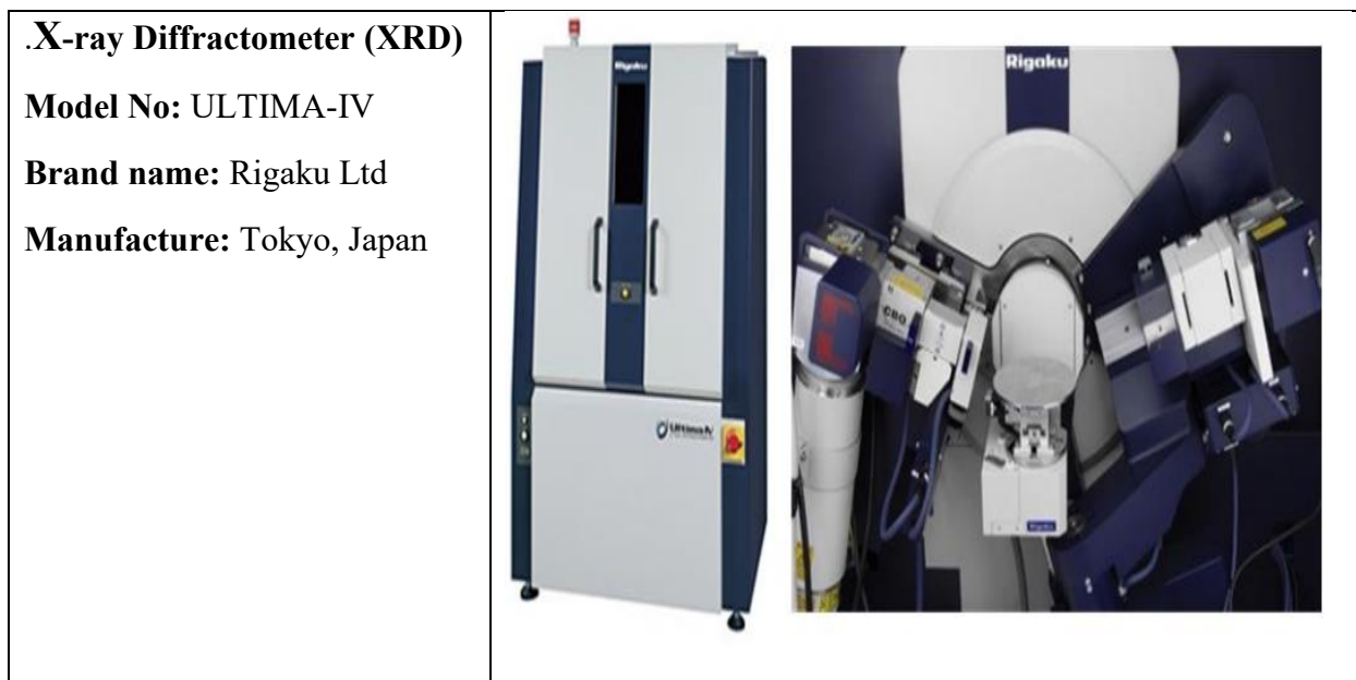
Figure 3. 10 An X-ray diffractometer is used to analyze the crystalline structure of jute fibres.
