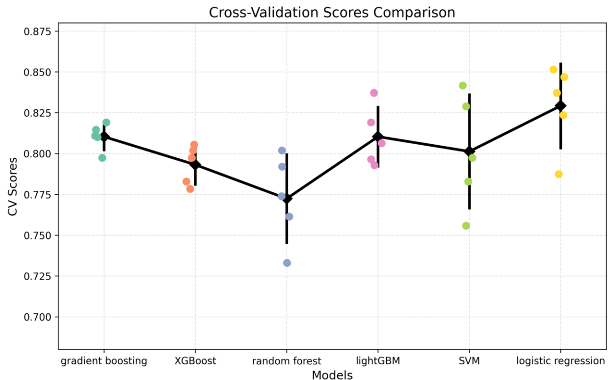
Figure 3.34: Cross validation of different ML models. Scatter plot comparing cross-validation scores across six machine learning models: gradient boosting, XGBoost, random forest, LightGBM, SVM, and logistic regression. Colored dots represent individual scores, while black lines with error bars indicate mean performance and variability. The visualization highlights model robustness and predictive accuracy for IBS-related classification tasks.
