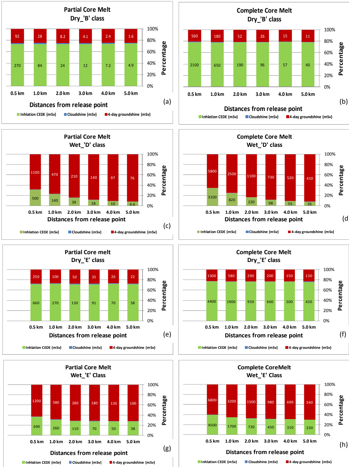
Figure 5-12: Three pathway contributions to TEDE for different stability classes (a & b) dry ‘B’ (c & d) wet ‘D’ (e & f) dry ‘E’ (g & h) wet ‘E’ in (a, c, e, g) PCM and (b, d, f, h) CCM states of LTSBO.
