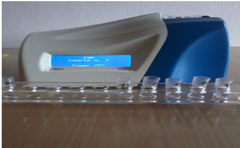
Image-1: Semi-automated ‘Turbiquick’ machine and Cuvette
