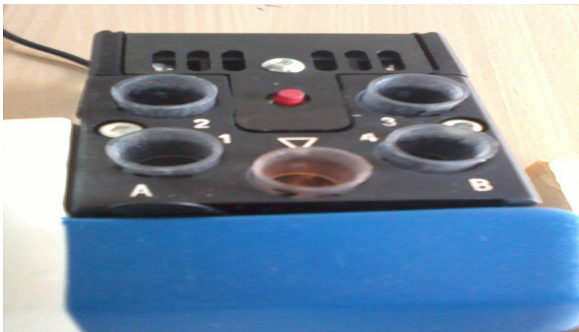
Image-3: One 'Pre-Incubation hole' (arrow) and 4 reading channels of the 'Turbi-quick machine'.
