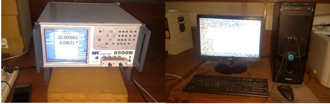
Figure 4.9: Wayne Kerr Impedance Analyzer [picture taken from Bangladesh Atomic Energy Centre, Dhaka]
