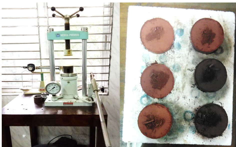
Figure 3.2: The preparation of palletized shape sample by hydraulic method in the Materials Science Division laboratory of Atomic Energy Centre, Dhaka (captured with permission).
