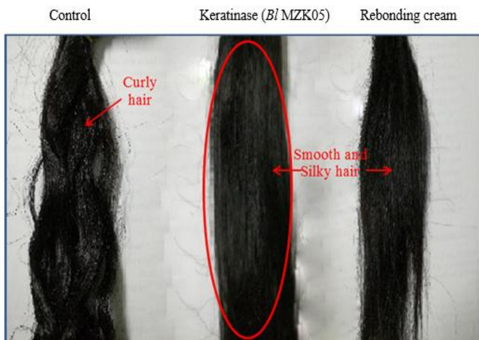
Figure 7.3.1: Hair rebonding test by recombinant keratinase
