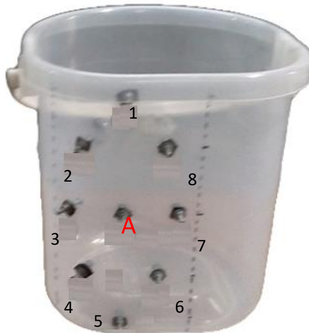
Figure5.77: Prepared Human Thorax Phantom.
