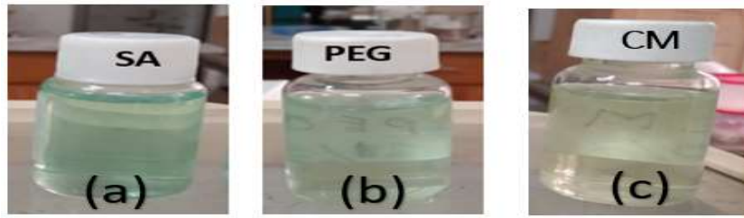
Fig 3.17: Visual representation of color removal by using (a) PSF-SA membrane (b) PSF-PEG membrane, and (c) commercial membrane
