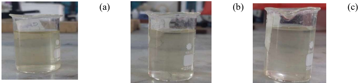
Fig 3.34: Visual representation of color removal by using (a) CM membrane (b) PES-PEG membrane, and (c) PES-PVP membrane
