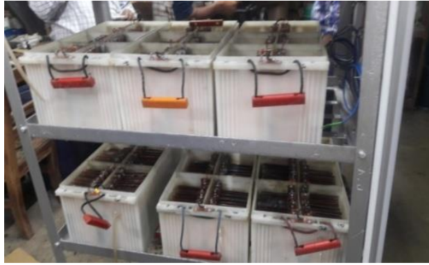
Figure 2.17: Fabrication of an experimental setup of a 1 KW PKL power production from the PKL/AL extract
