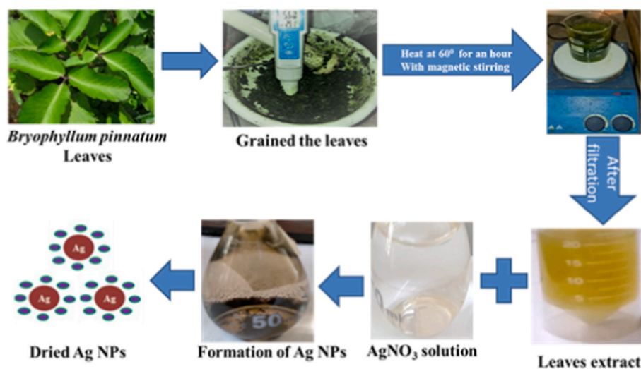
Fig. 1. Steps diagram of green synthesis of AgNPs using Bryophyllum pinnatum leaves extract. (For interpretation of the references to color in this figure legend, the reader is referred to the Web version of this article.)
