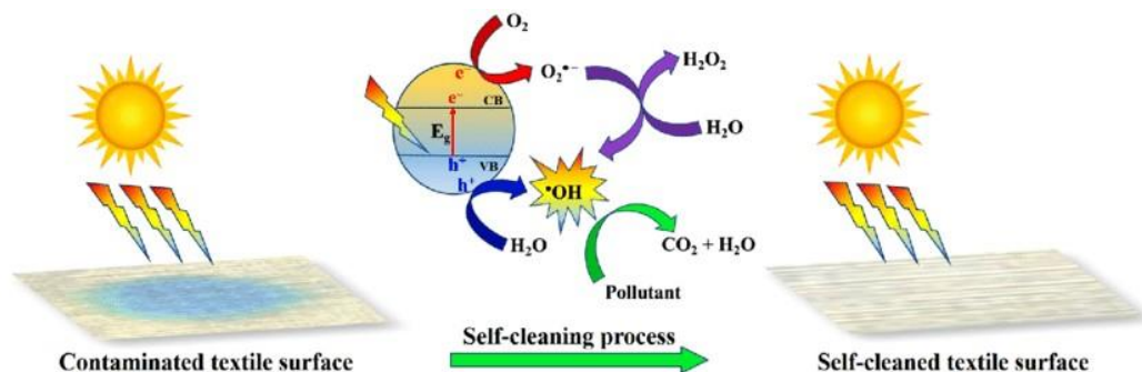
Figure 1.8: Self-cleaning mechanism based on photocatalytic degradation of TiO 2 coated cotton. 51
