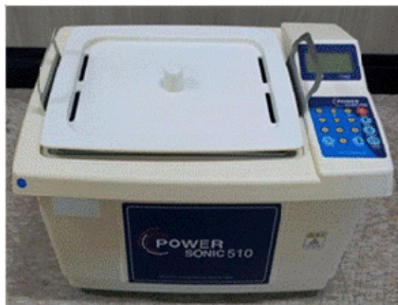
Figure 3.9: Ultrasonicator of Model no Power sonic 510, Hwa Shin Technology, SEOUL, KOREA, having frequency- 50 Hz, Input voltage- 230AC, Output power-500W.
