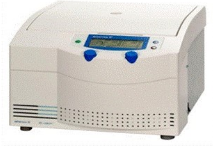
Figure 3.7: Centrifuge machine of Model: Sigma 2-16 P, Speed: 15000 rpm (max), Company: SIGMA Laborzentrifugen, Country: Germany, situated in Atomic Energy Centre Dhaka.
