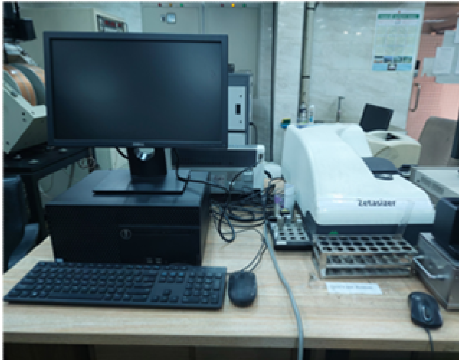
Figure 3.18. Dynamic light scattering instrument of model: ZEN3600, RatedVoltage: AC 100-240 V, Rated frequency: 50/60 Hz, Rated Input Power: 250 V, Company: MALVERN INSTRUMENTS LTD, Country: UK.
