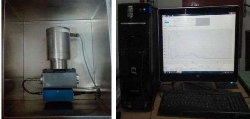
Figure 3.14: Mössbauer spectroscopy of Resonant Gamma-Ray Spectrometer, Model: W302, Company: WEB RESEARCH CO, Country: USA.
