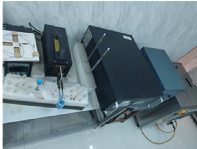
Figure 3.21: Hyperthermia Set-up Material Science Division, Atomic Energy Centre, Dhaka, Model: EASY HEAT 5060LI, Input voltage: 187-265 AC, Frequency: 150-400 Hz, In-Out power: 3 Kw-60 Kw, Company: Ambrell, USA.
