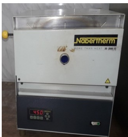
Figure 3.6: Oven for sample heat treatment of Model L3/12/C6, Lilienthal, Germany.
