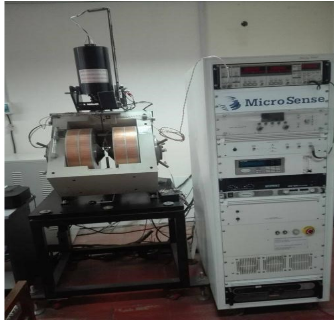
Figure 3.12: Vibrating sample magnetometer of Model: EV-9 (3473-70 electromagnet), Temperature range: -170^{\circ}\text{C} - 700^{\circ}\text{C} , Magnetic field: 2.1 Tesla, Max.), Company: Microsense L.L.C., Country: USA situated in Atomic Energy Centre Dhaka.
