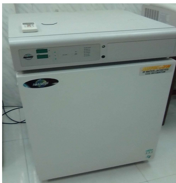
Figure 3.23: Co 2 Incubator (Nuair, U.S.A) in the cell culture lab
