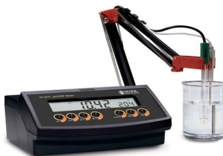
Figure 3.3: The pH meter of the model was HI 2211, HANNA Instruments, Europe, Romania. Model no of the pH probe was HI 7662, HANNA, Romania.
