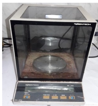
Figure 3.4: Balance meter of model SP250, SCIENTECH BOULDER CO, U.S.A.
