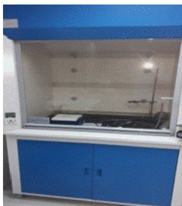
Figure 3.5: Fume hood of model FH 1200(E), JINAN BIOBASE BIOTECH CO.LTD., China.
