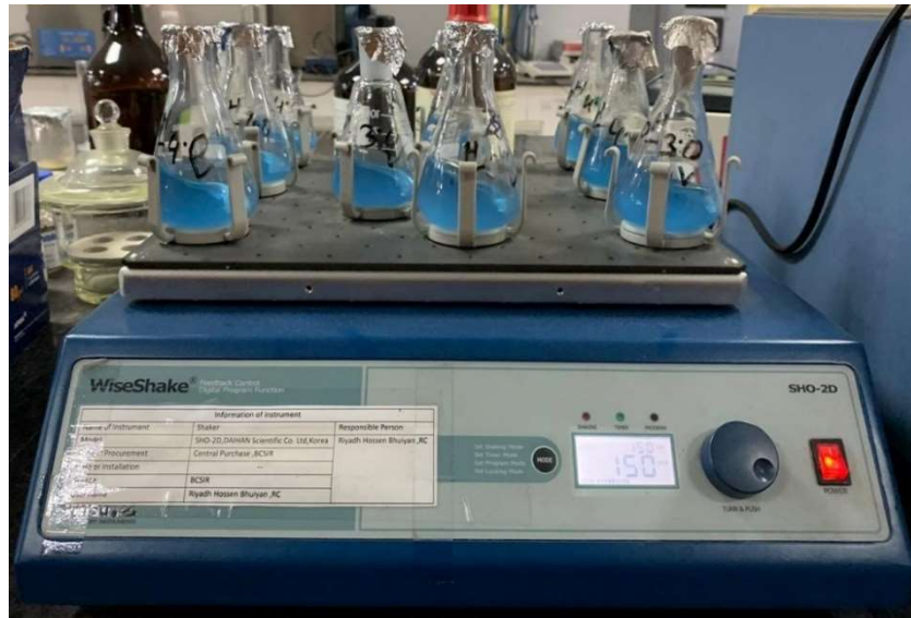
Figure 3.1 Shaking of aqueous solution with the help of Orbital Shaker.
