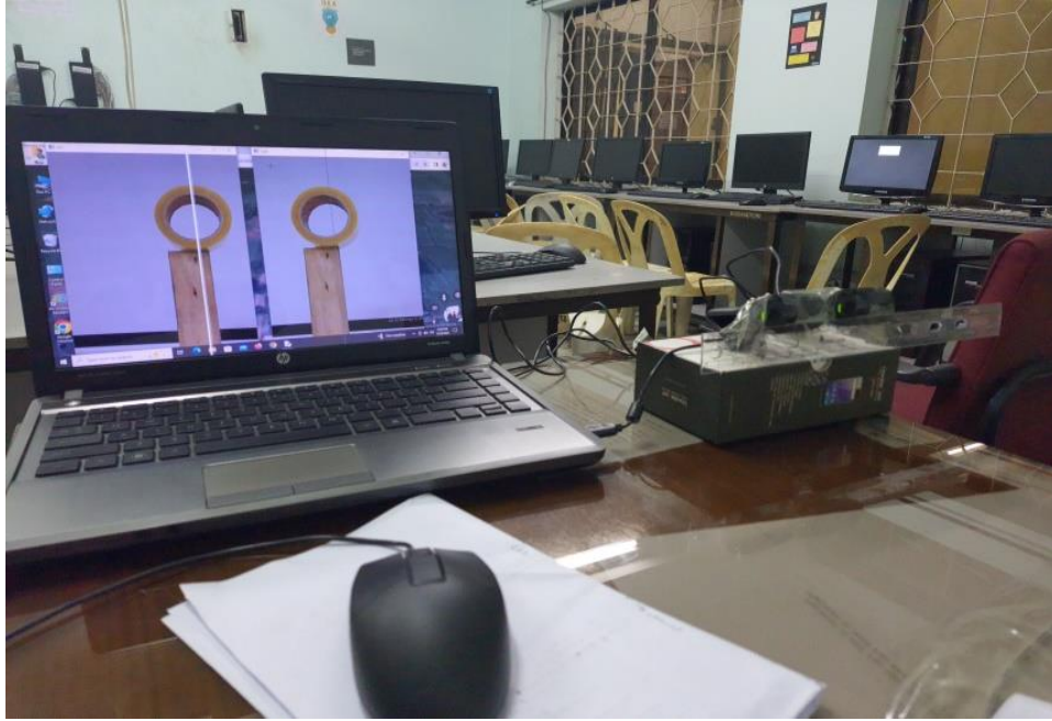
c) Real image acquisition using stereo web camera for dataset-3(Scotch tape stand).
