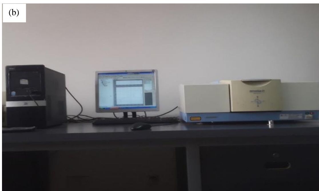
Figure 3.10: (a) Schematic illustration of an FTIR spectrometer. Adapted from [189] and (b) Photograph of the SHIMADZU FTIR spectrophotometer (IR Prestige-21).
