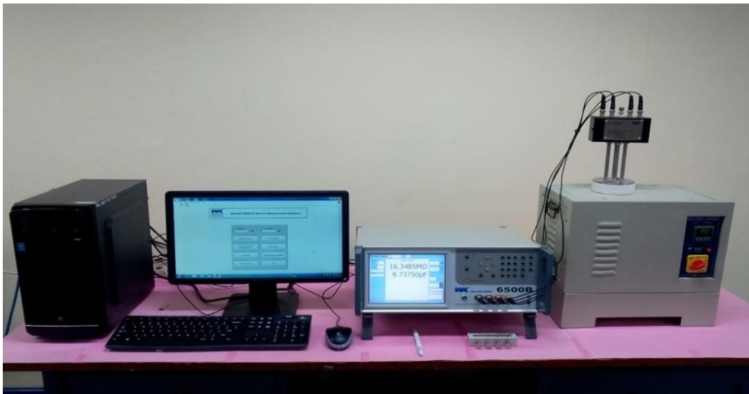
Figure 3.13: Photograph of precision impedance analyzer (Wayne-Kerr, Model: 6500B)
