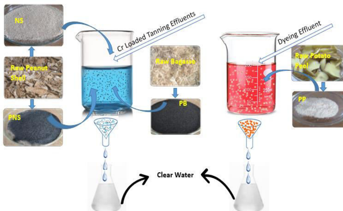
Figure 2.6 Schematic set up of an adsorption process
