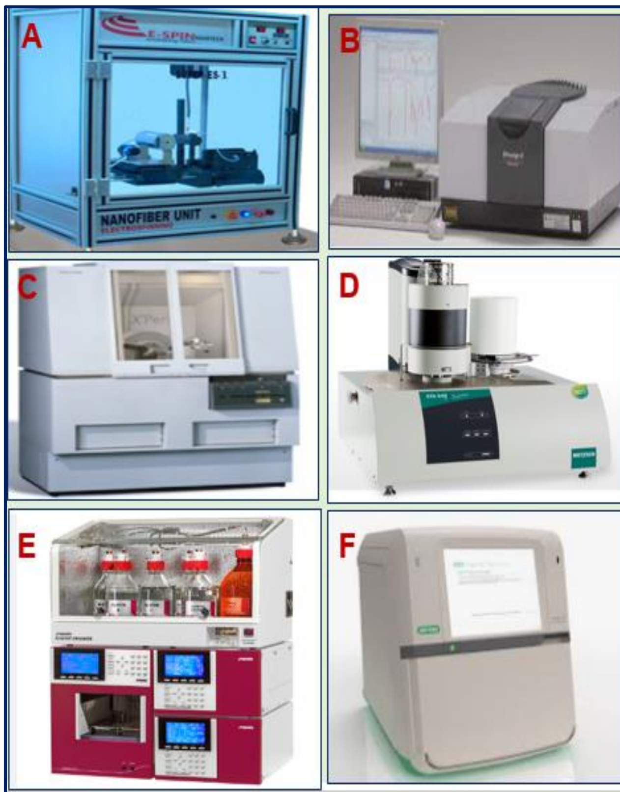
Figure 2.1 Instruments used for the study (A) Electro spinneret, (B) FT-IR spectrometer, (C) X-ray diffractometer, (D) Thermal analyzer, (E) Amino acid analyzer, (F) Gel electrophoretic system
