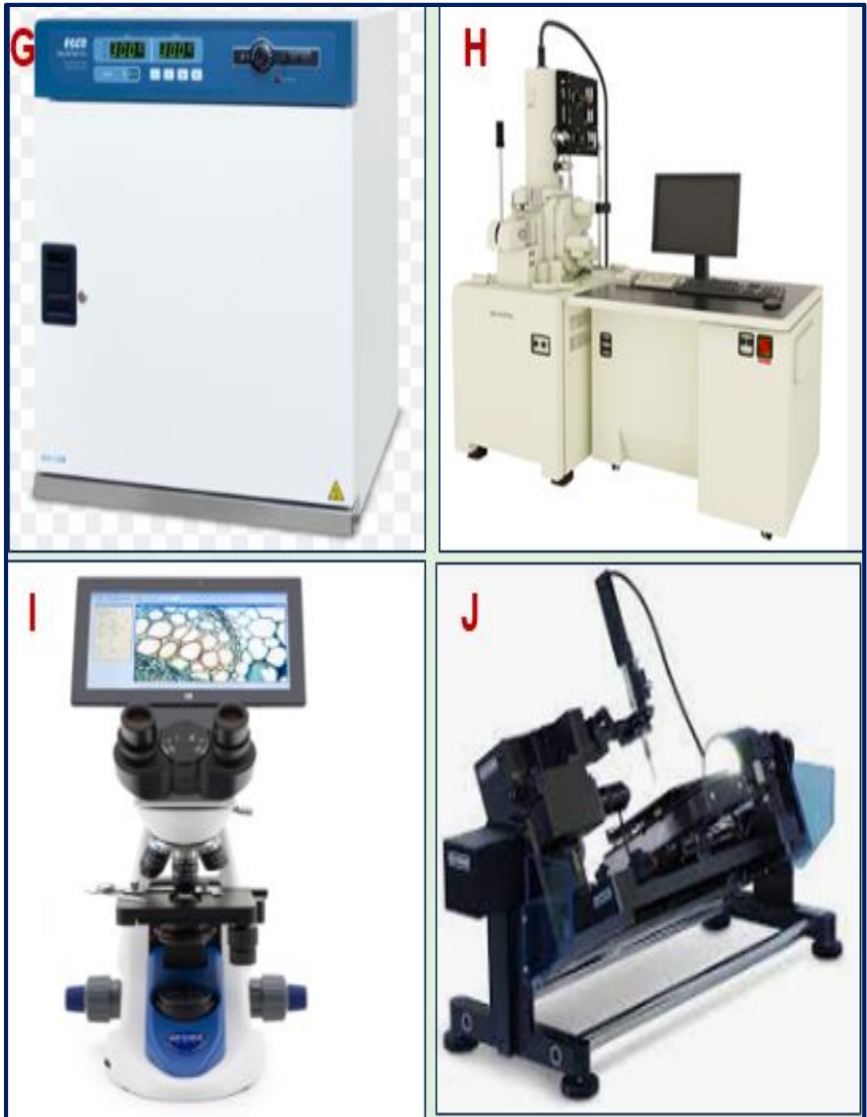
Figure 2.2 Instruments used for the study (G) Oven, (H) FESEM, and (I) Optical Microscope, (J) Contact angle analyzer
