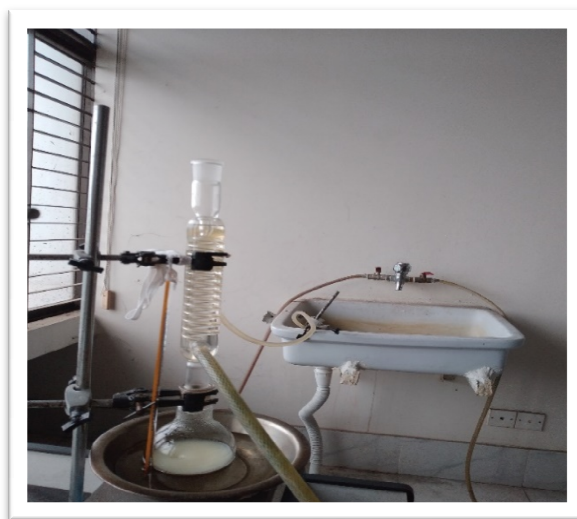
Figure 2.1. A set of equipment, used for the synthesis of antibiotic-metal complexes.
