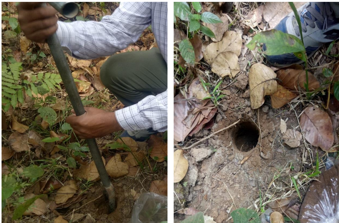
Figure 3.12: Photos showing the procedure of soil collection.
