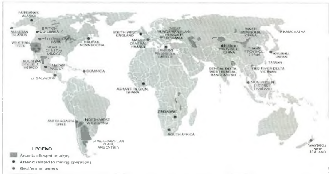
Fig. 7: Distribution of documented arsenic problems in groundwater major aquifers as well as water and environmental problems related to mining and geothermal sources. Areas in blue are lakes 84 .
