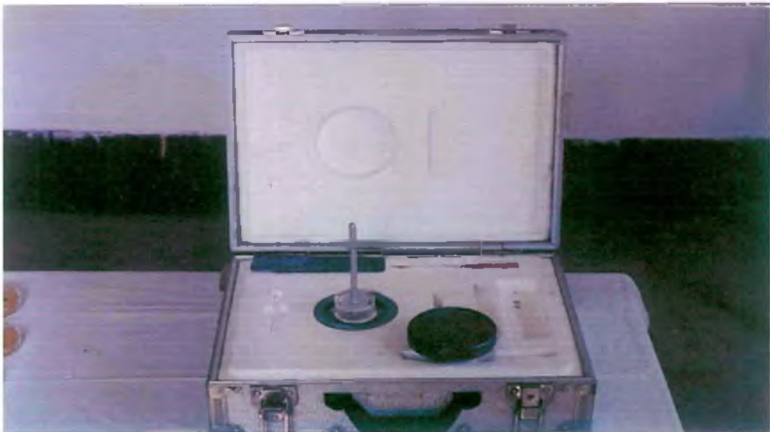
Fig.17: Beta Applicator ( ^{90}\text{Sr} ) employed for the present study.
